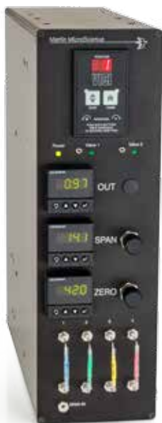
The MMSD-MPV System is a low volume dilution apparatus with a clearing time of less than five minutes and all wetted parts are constructed of stainless steel that is capable of dilution ratios as low as 1:10,000.
